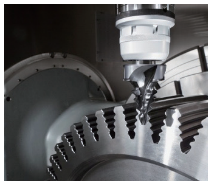
图9 榫槽铣削加工 Fig.9 Trochoidal milling of fir-tree slot
