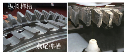
图10 线切割加工榫槽 Fig.10 WEDM of fir-tree root slot
