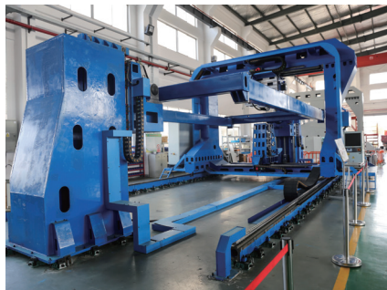
图7 上海拓璞数控中央翼自动钻铆设备 Fig.7 Central wing panel machine developed by TOPNC
