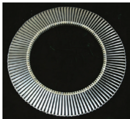
图4 \gamma -TiAl合金低压涡轮叶片 Fig.4 Low pressure turbine blades of \gamma -TiAl alloy
