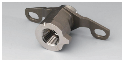
图3 MTU公司采用SLM技术制造管道镜套筒 Fig.3 MTU testing component made by SLM process
